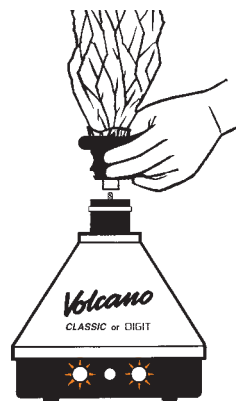
Attach valve balloon to filling chamber
