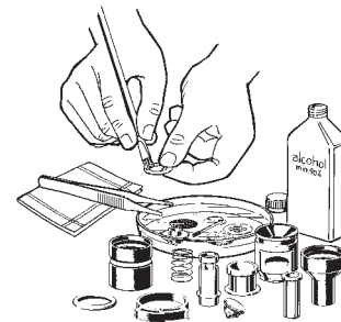
Manual cleaning with alcohol (min. 90%)
