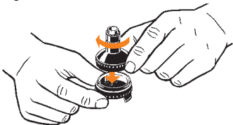
Screw on filling chamber cap
